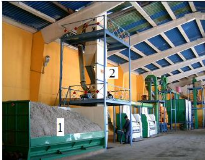
1-UPS type hair seed receiving and transmitting device, 2-ChSA type seed sorting unit. Figure 5. Photo of hairy seed preparation technology.
