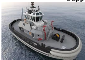
tugboat – maneuvers other vessels by pushing or pulling them
